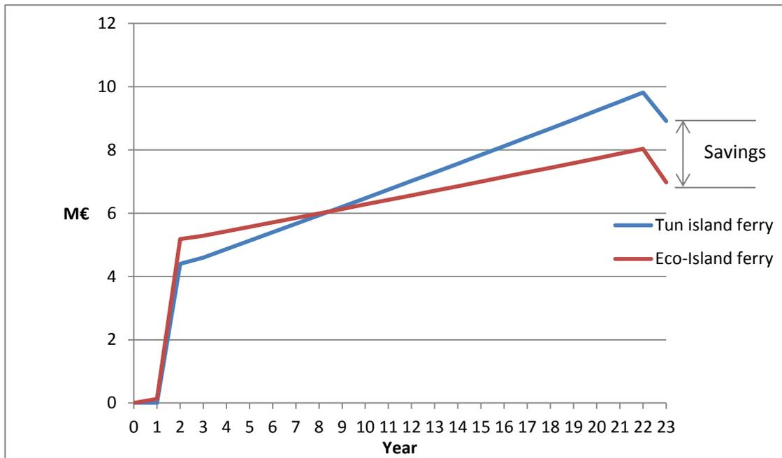
**Figure 10 Accumulation of costs at present value with 3 return trips per day**
