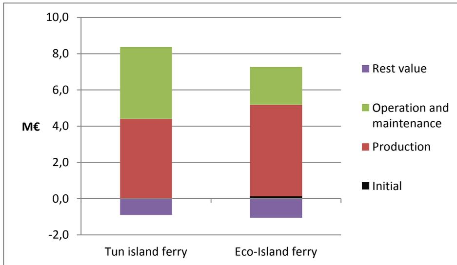
**Figure 8 Contribution from different phases in the life cycle cost, presented at present value**
