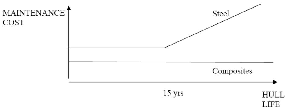
**Figure 4 Illustration of maintenance costs over time**
